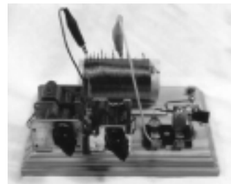
The completed high performance crystal set with IN34A diode installed in detector clips for testing operation.
